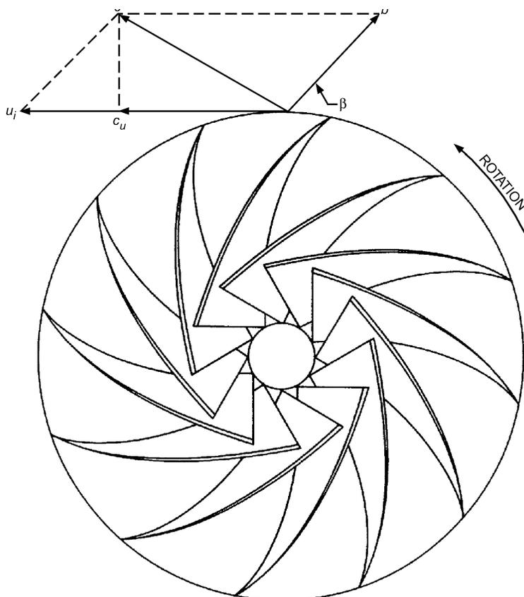
Fig. 20 Impeller Exit Velocity Diagram
