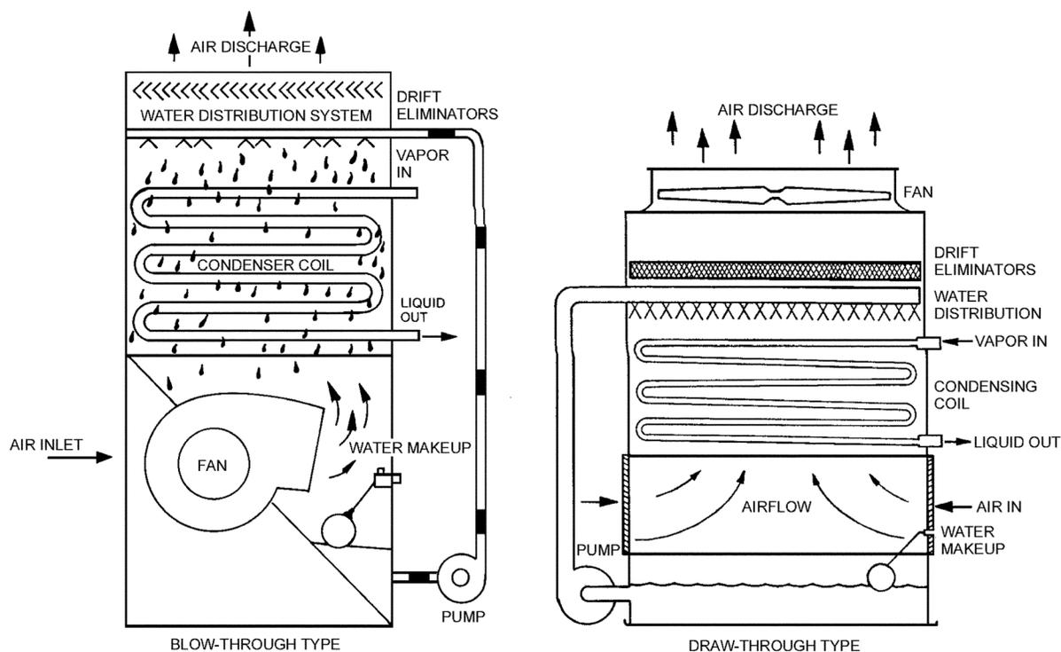
Fig. 24 Functional View of Evaporative Condenser
