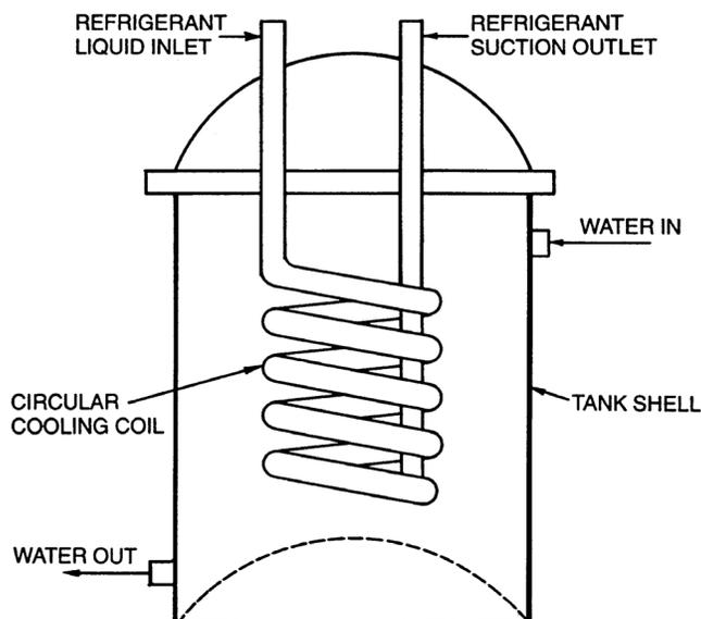
Fig. 37 Shell-and-Coil Cooler
