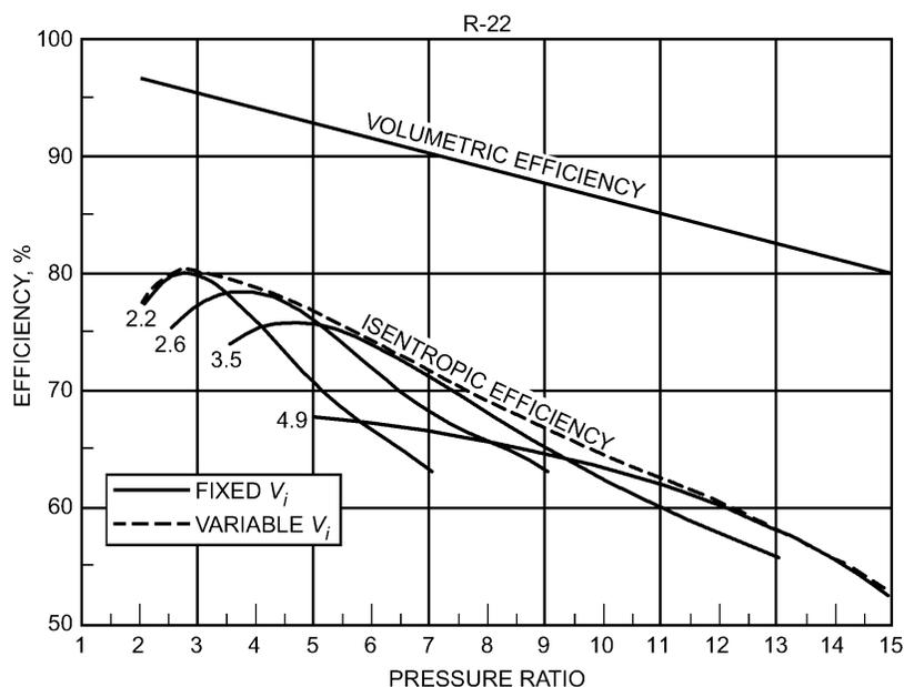
Fig. 11 Typical Screw Compressor Performance with R-22
