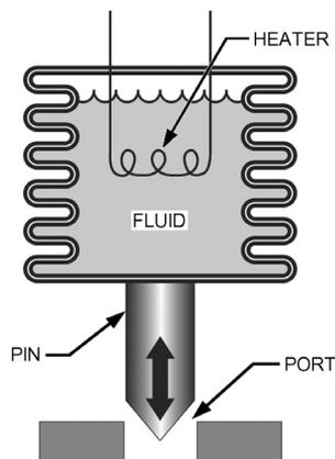
Fig. 29 Fluid-Filled Heat-Motor Valve (Figure 20, Chapter 11, 2018 ASHRAE Handbook—Refrigeration)
