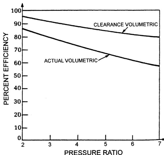
Fig. 5 Volumetric Efficiency
