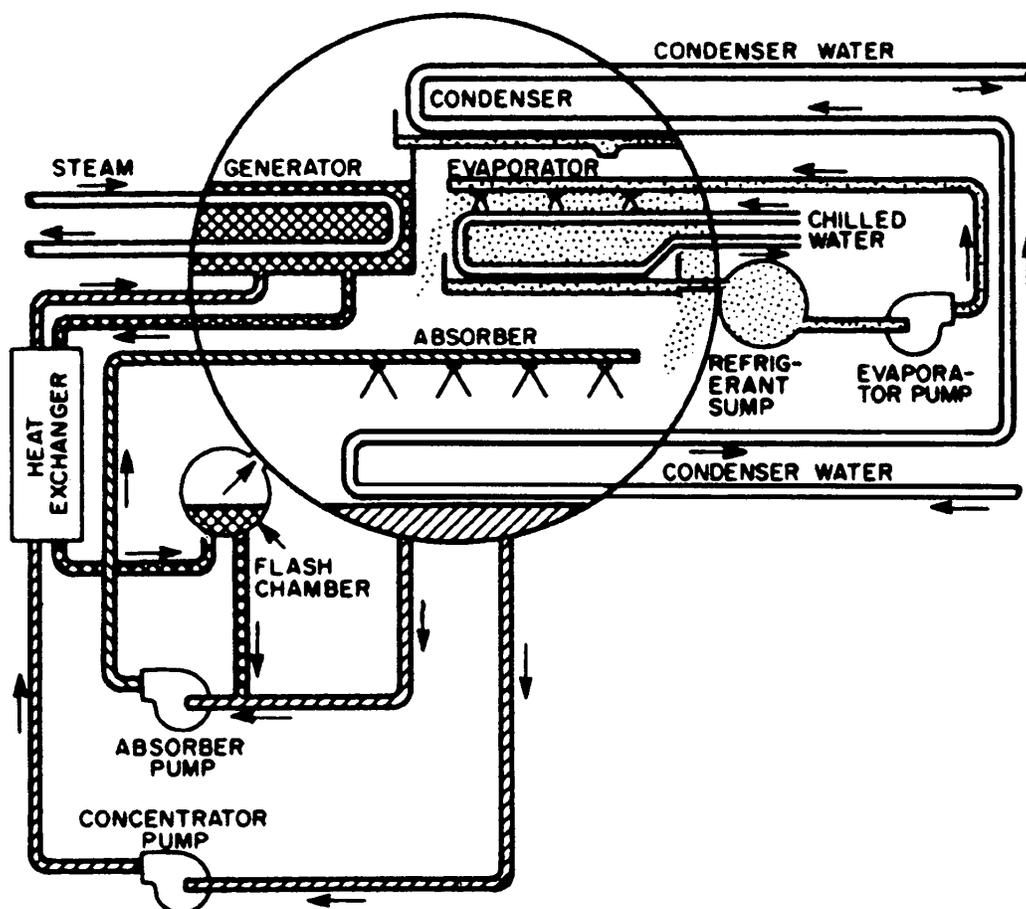
Fig. 39 Diagram of One-Shell Lithium Bromide Cycle Water Chiller
