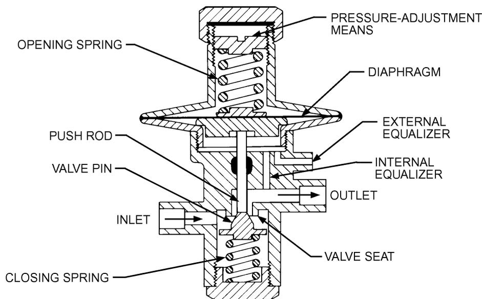
Valve is used with either internal or external equalizer, but not with both.
