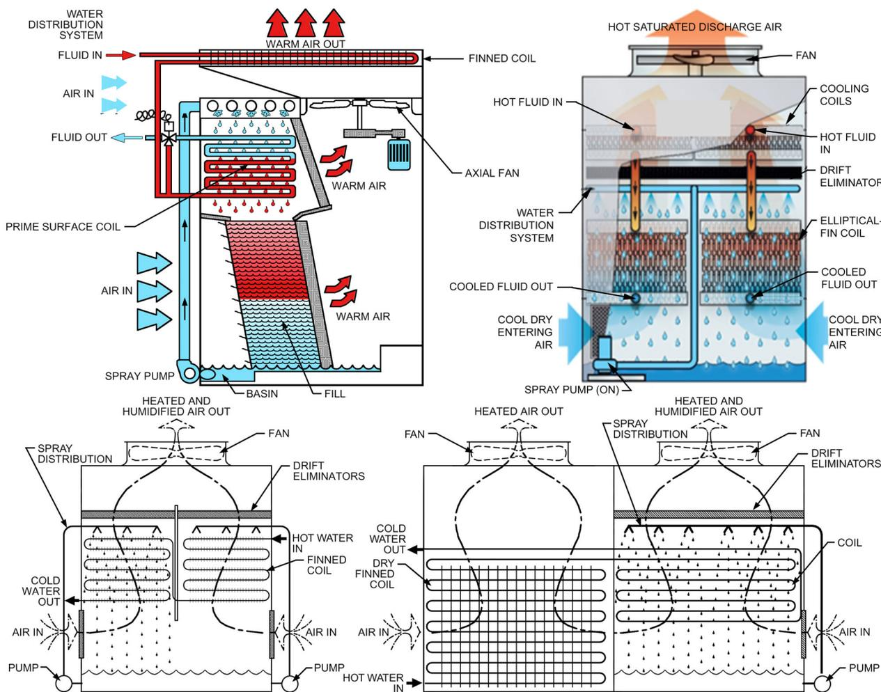
Fig. 42 Counterflow Forced-Draft Cooling Tower
