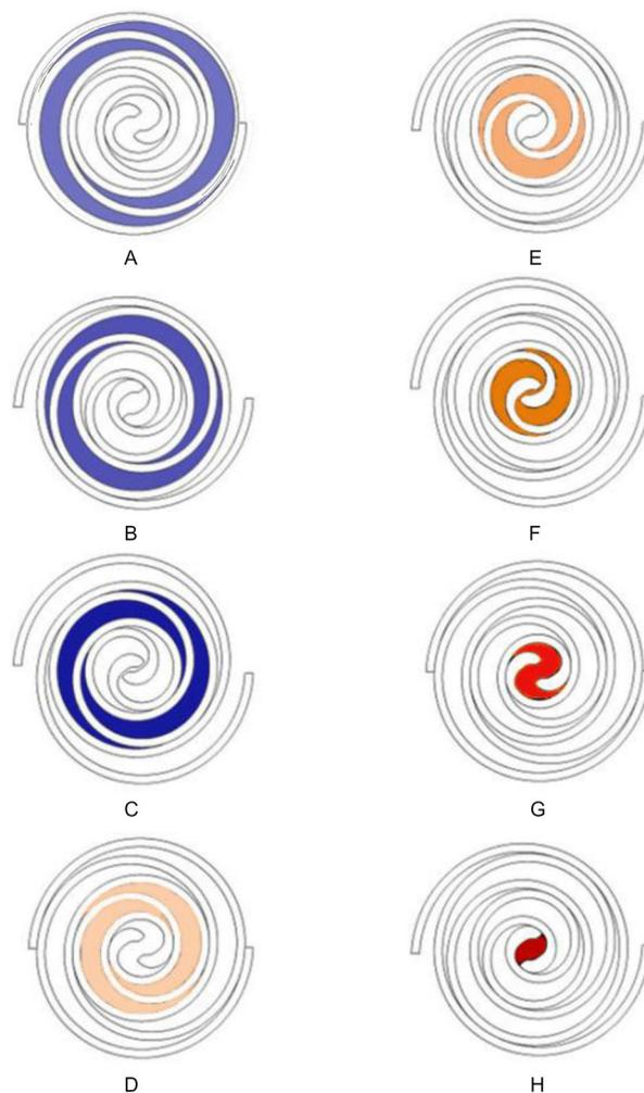
*Fig. 15 Scroll Compression Process*
