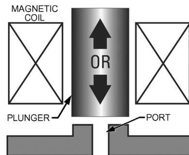
Fig. 31 Pulse-Width-Modulated Valve (Figure 22, Chapter 11, 2018 ASHRAE Handbook—Refrigeration)
