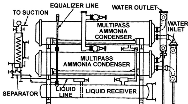
Fig. 22 Horizontal Shell-and-Tube Ammonia Condenser and Receiver
