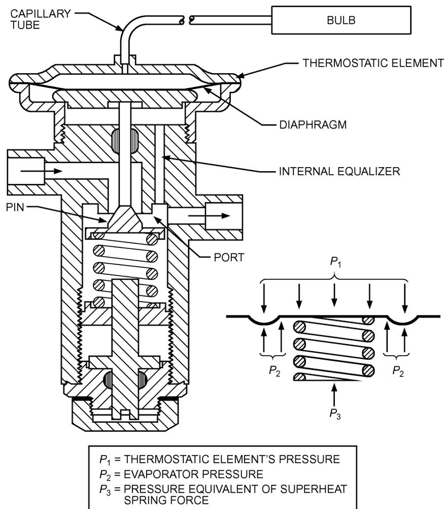
Fig. 25 Typical Thermostatic Expansion Valve
