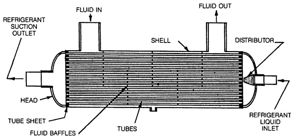
Fig. 36 Direct-Expansion Shell-and-Tube Cooler
