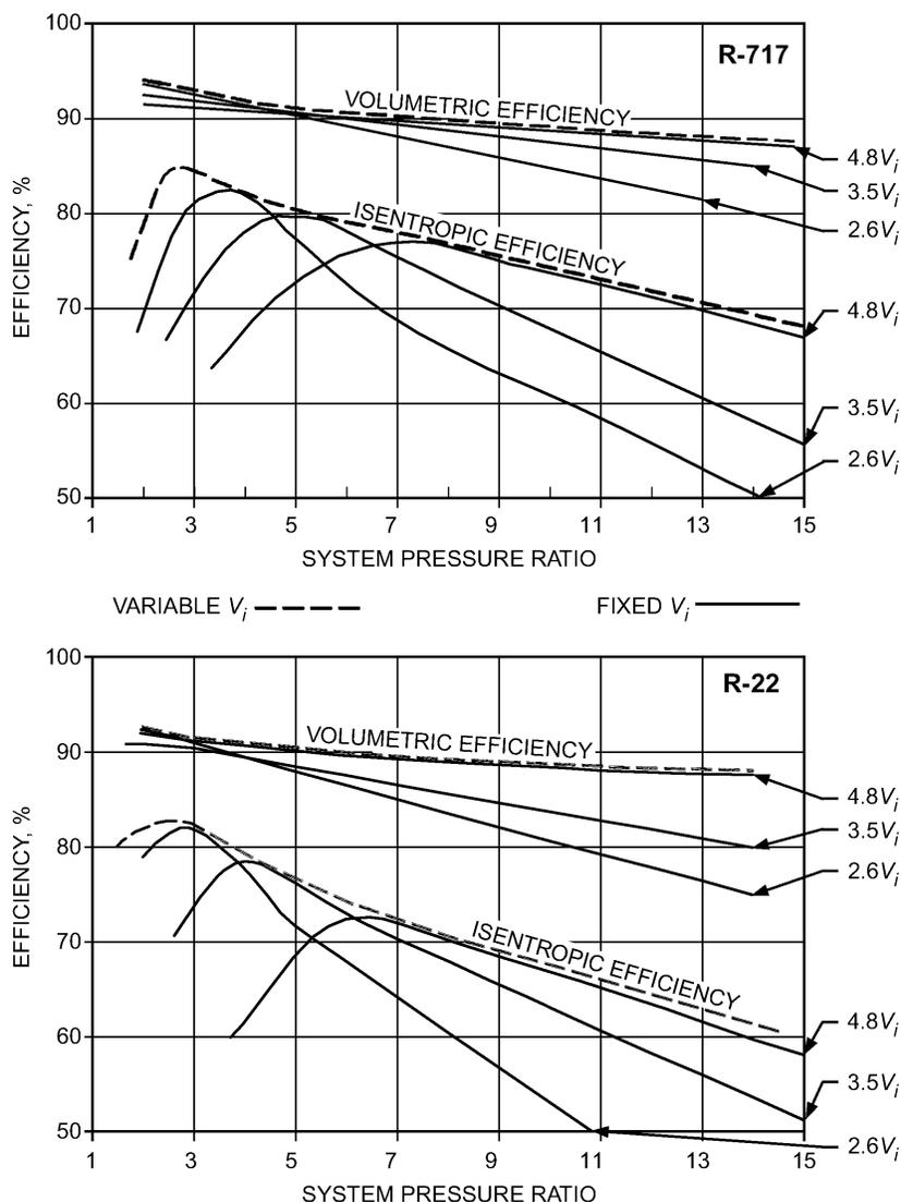
Fig. 14 Twin-Screw Compressor Efficiency Curves
