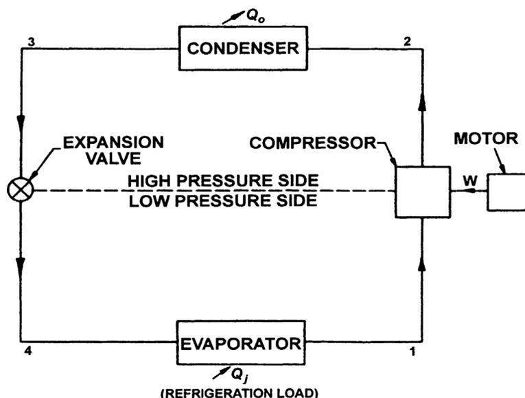
Fig. 1 Simplified Equipment Diagram for the Basic Vapor-Compression Cycle
