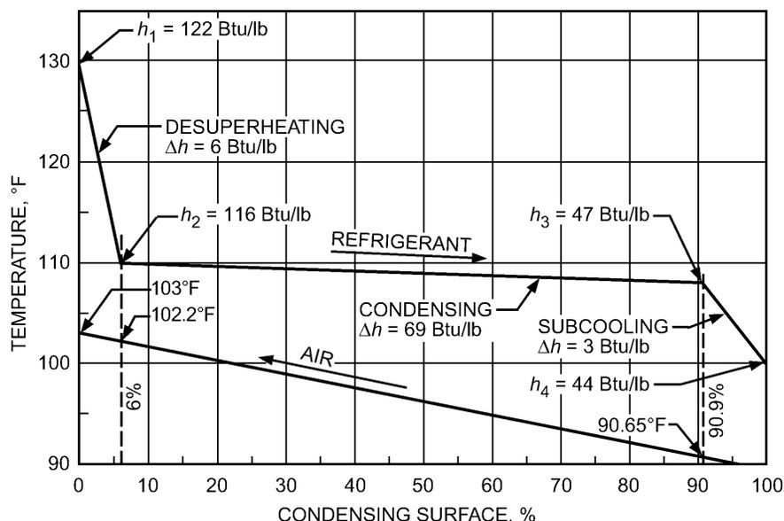
Fig. 23 Temperature and Enthalpy Changes in Air-Cooled Condenser with R-134a
