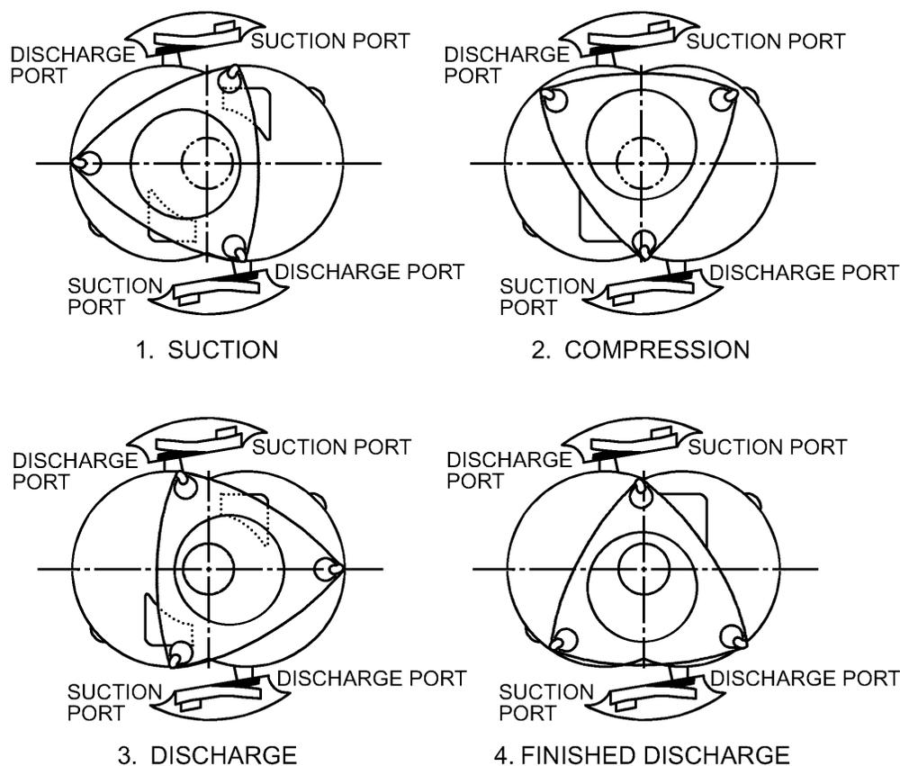
Fig. 18 Sequence of Operation of Wankel Rotary Compressor
