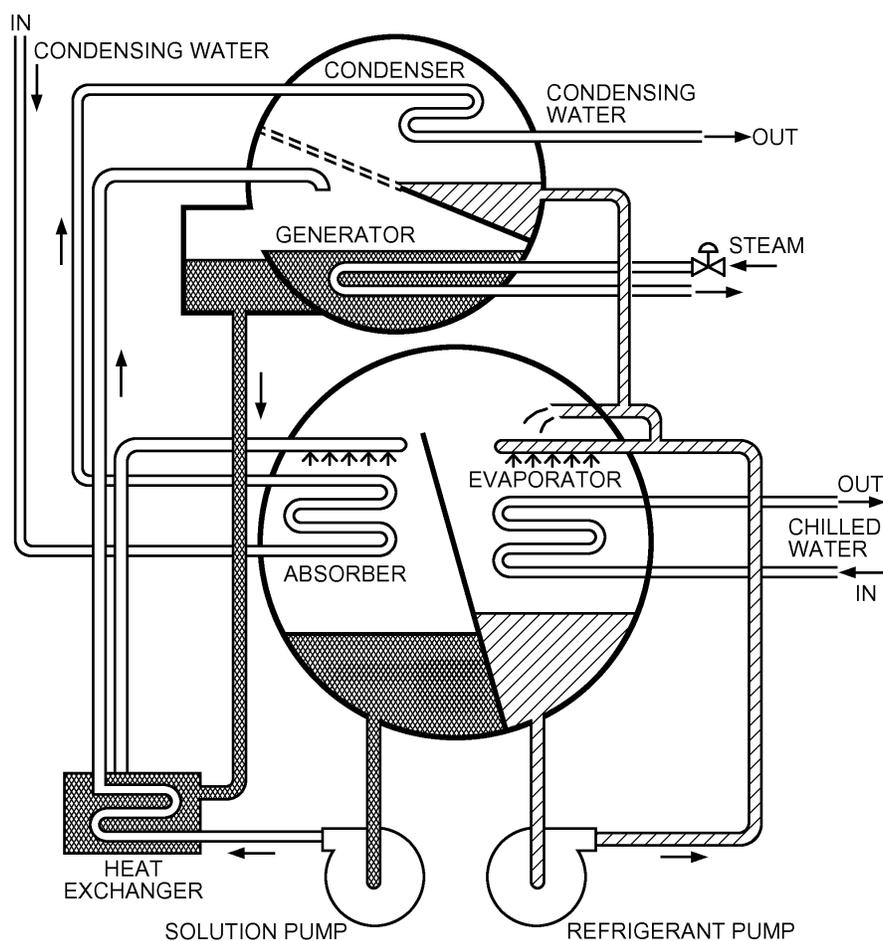
Fig. 38 Two-Shell Lithium Bromide Cycle Water Chiller
