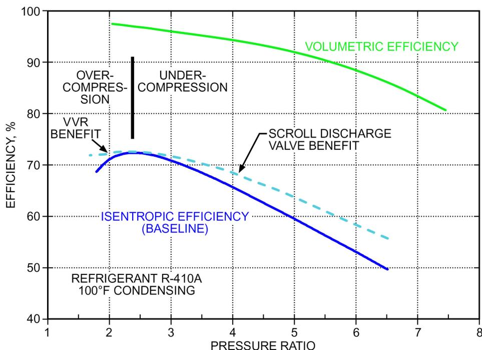
Fig. 16 Volumetric and Isentropic Efficiency versus Pressure Ratio for Scroll Compressor (Figure 49, Chapter 38, 2020 ASHRAE Handbook—HVAC Systems and Equipment)
