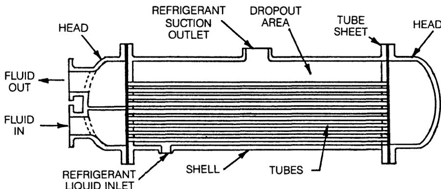
*Fig. 35 Flooded Shell-and-Tube Cooler*
