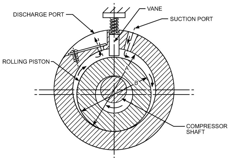
Fig. 6 Fixed-Vane Rolling Piston Rotary Compressor
