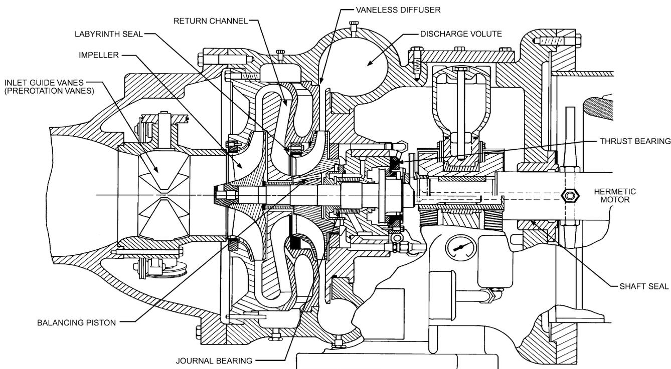
Fig. 19 Centrifugal Refrigeration Compressor
