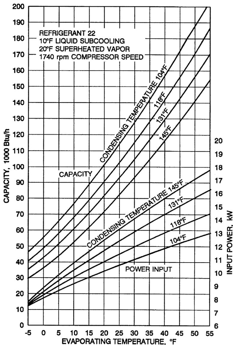
Fig. 3 Typical Capacity and Power for Reciprocating Compressor (Figure 10, Chapter 38, 2020 ASHRAE Handbook—HVAC Systems and Equipment)
