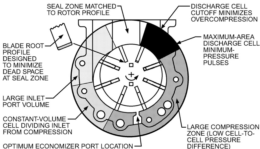
Fig. 7 Rotary Vane Compressor
