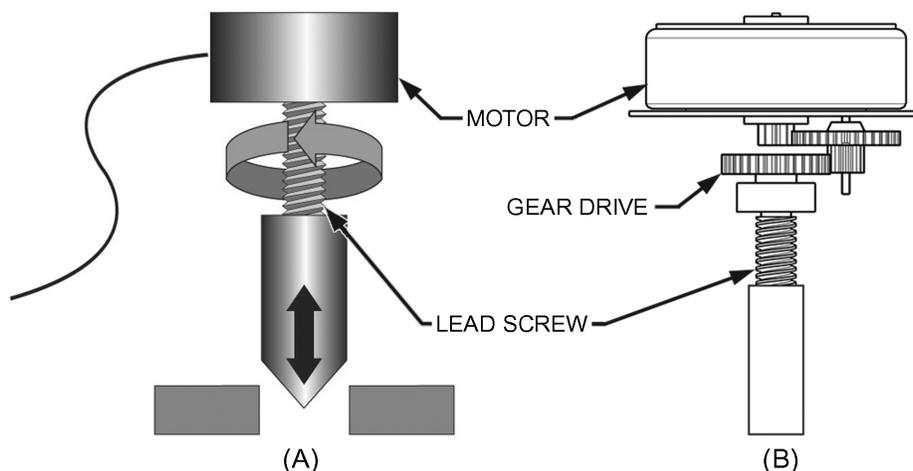
Fig. 32 Step Motor with (A) Lead Screw and (B) Gear Drive with Stem Seal (Figure 23, Chapter 11, 2018 ASHRAE Handbook—Refrigeration)
