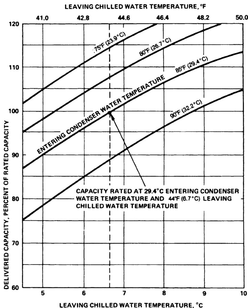
Fig. 41 Performance Characteristics of Lithium Bromide Cycle Water Chiller
