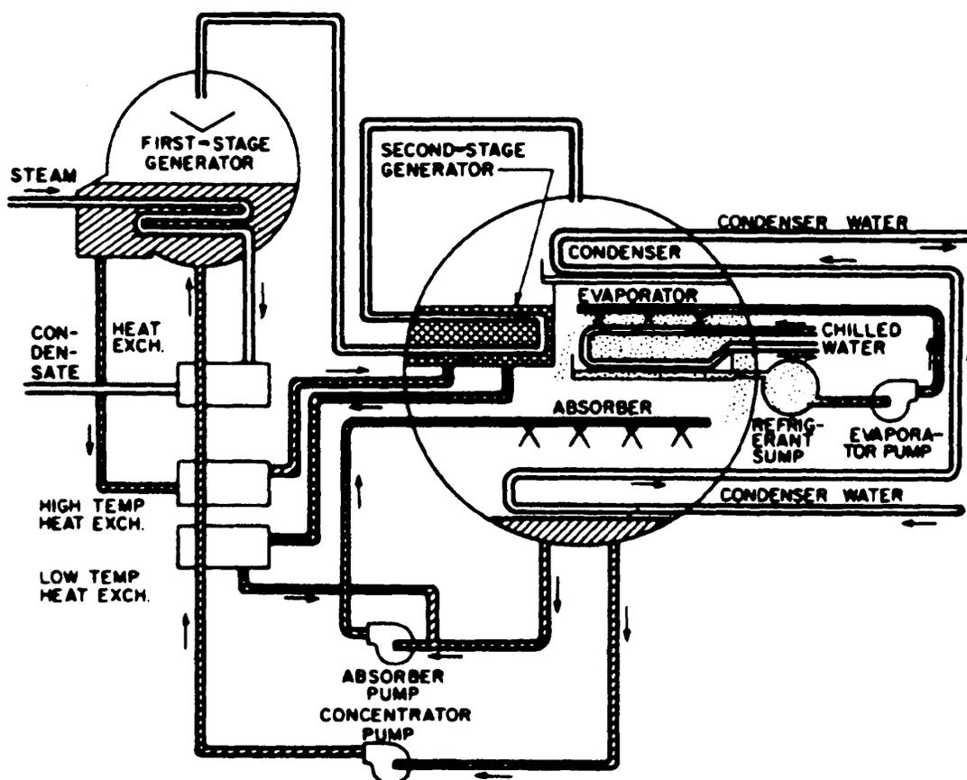
Fig. 40 Diagram of One-Shell Lithium Bromide Cycle Water Chiller with Two-Stage Generator
