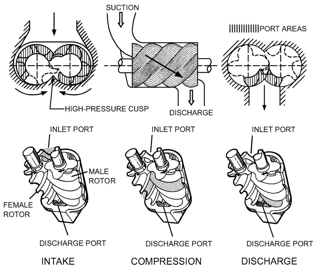
Fig. 13 Twin-Screw Compressor
