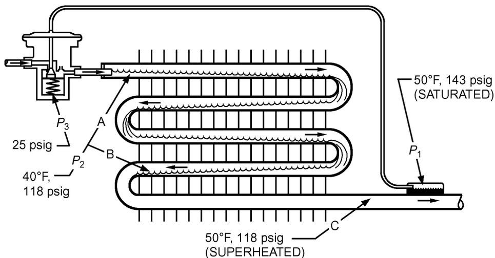
Fig. 26 Thermostatic Expansion Valve Controlling Flow of Liquid R-22
