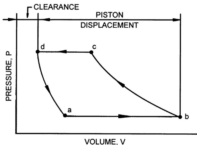
Fig. 4 Cycle for Idealized Piston Compressor
