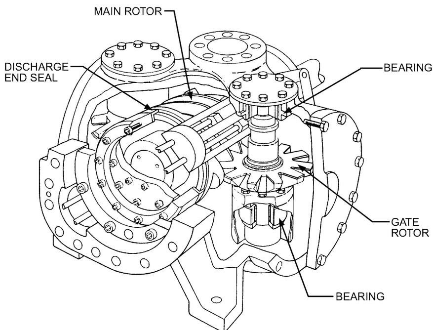
Fig. 9 Section of Single-Screw Compressor
