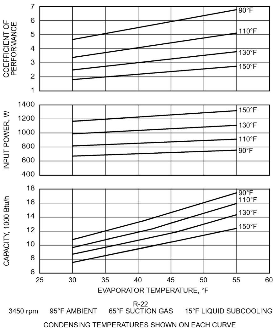
Fig. 8 Typical Rolling Piston Compressor Performance
