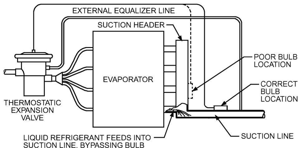
Fig. 27 Bulb Location for Thermostatic Expansion Valve
