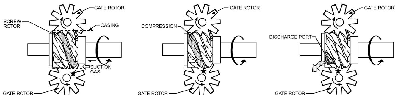
**Suction.** During rotation of the main rotor, a typical groove in open communication with the suction chamber gradually fills with suction gas. The tooth of the gaterotor in mesh with the groove acts as an aspirating piston.
