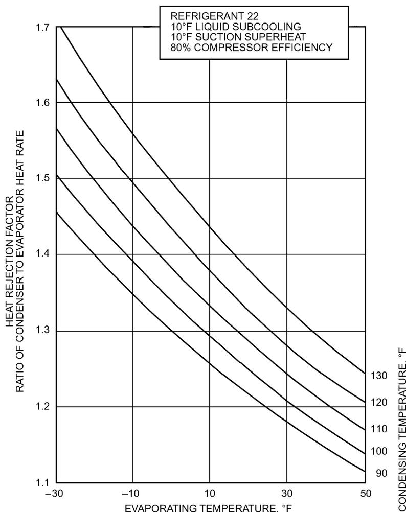
Fig. 21 Heat Removed in Condenser
