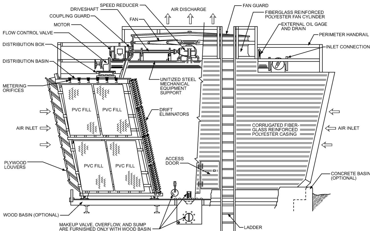
Fig. 43 Crossflow Induced-Draft Tower
