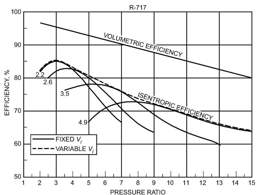
Fig. 12 Typical Screw Compressor Performance with R-717 (Ammonia)
