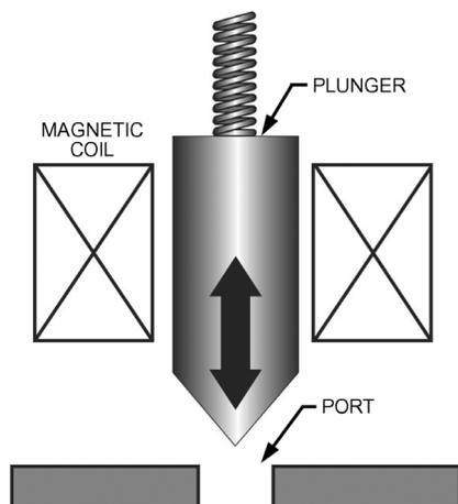
Fig. 30 Magnetically Modulated Valve (Figure 21, Chapter 11, 2018 ASHRAE Handbook—Refrigeration)
