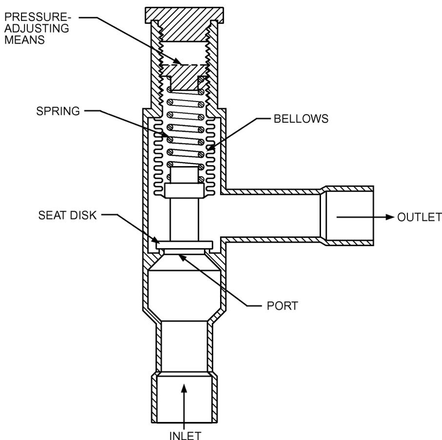
Fig. 33 Direct-Acting Evaporator Pressure Regulator
